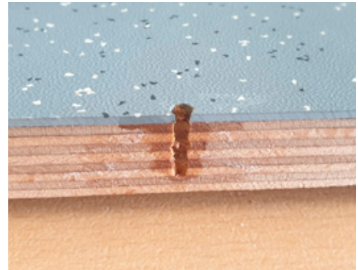
Non-impregnated borehole after water ingress
